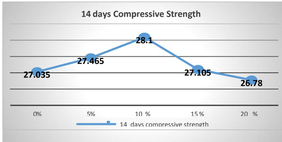
Fig. 2: 14 Days Compressive Strength Test Results
