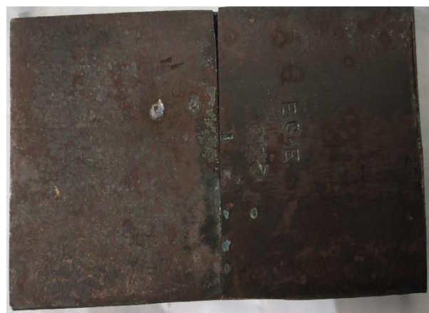
Fig. 2: Welded specimen before HT
