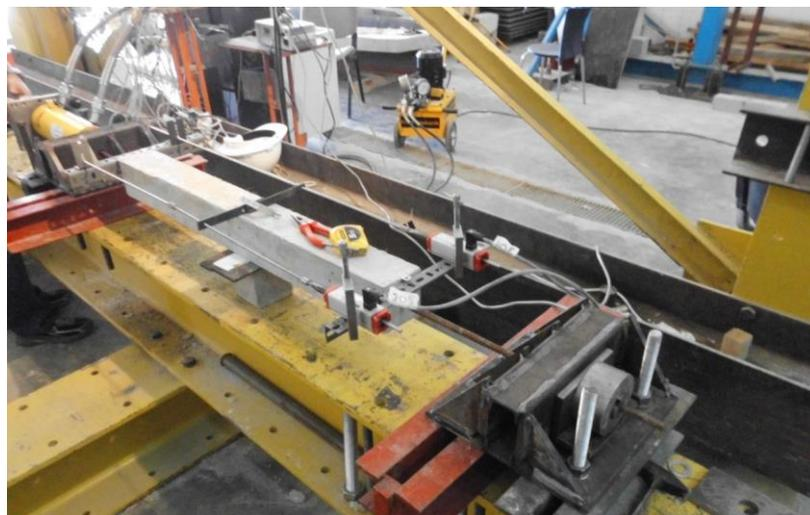
**Fig. 4: General view of prismatic tension specimens with reinforcing bar**
