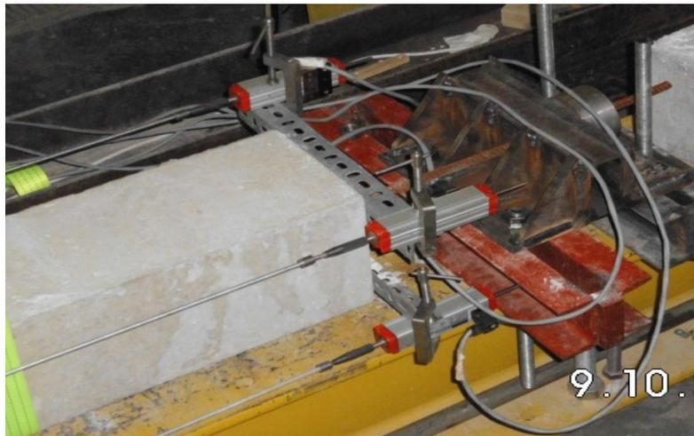
**Fig. 9:** Test set-up for prismatic tension specimens with bar - end 2 (displacement transducers)
