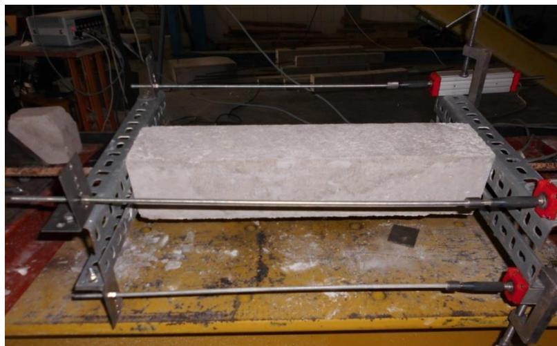
**Fig. 10:** Test set-up for prismatic tension specimens with bar
