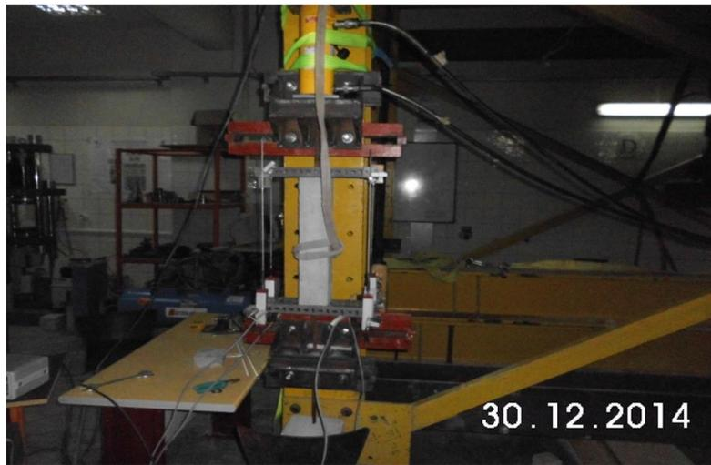
Fig. 11: Test set-up for prismatic tension specimens with bar (vertical direction)
