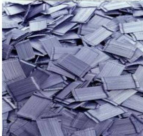
**Fig. 5: Dramix ZP 305 steel fiber used in the research**
