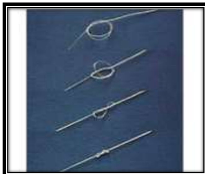
Fig. 9: A smart suture shrinks and tightens the knot when the temperature is raised above the thermal transition temperature
