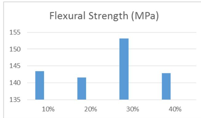
Fig 4.2 Flexural Strength Properties of 10%, 20%, 30% & 40% (KMnO<sub>4</sub>) Treated fibre composites
