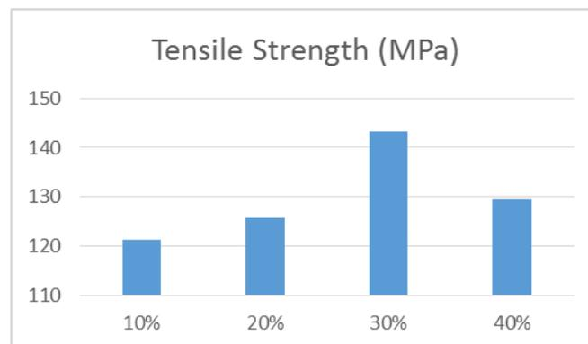
**Fig 4.1 Ultimate Tensile Strength of 10%, 20%, 30% & 40% (KMnO<sub>4</sub>) Treated fibre composites**
