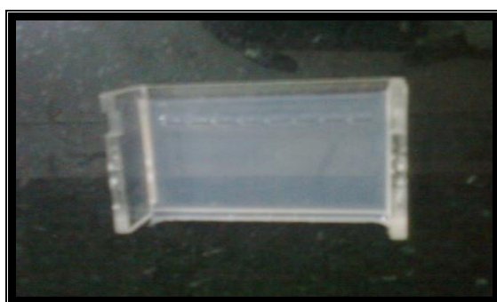
Fig 13: Gel was molted ethidium bromide added and casted in a casting tray having combs
