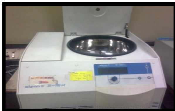
Fig 9: Centrifuge was taken to separate chemicals and cell extracts
