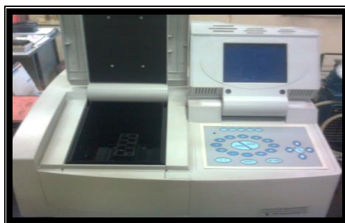
Fig 17: Concentration of isolated DNA was measured by U.V/ Visible Spectrophotometer
