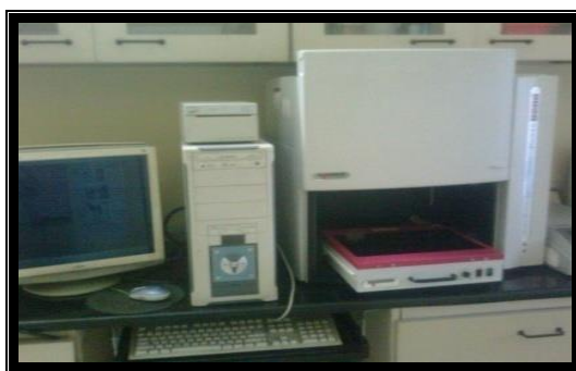
Fig 16: Gel documentation system was used to analysed the gel slab
