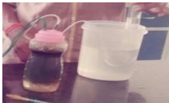
Figure 3: Hydrogen measuring instrument
