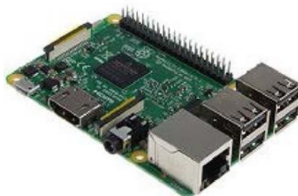
Fig.2. Raspberry Pi 3 Model B
