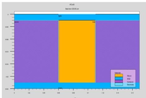
Fig 1(a.): Double Gate Simulated Structure
