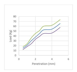
CBR value after flooding for 2.5 mm penetration: 3.43
