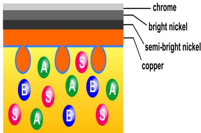
**Fig.3. Plastic Chrome Plating Structure**
