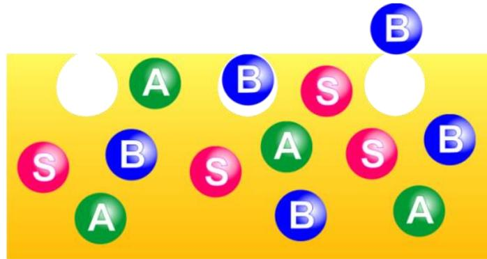
**Fig.2. Composition of Plastic for Chrome Plating**
