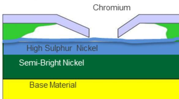
Fig.4. Corrosion Mechanisms of Nickel Layers
