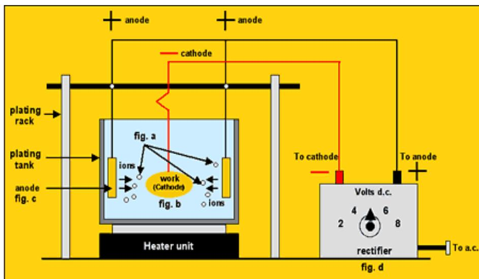
Fig.1. Simple Schematic Diagram of Electroplating Process
