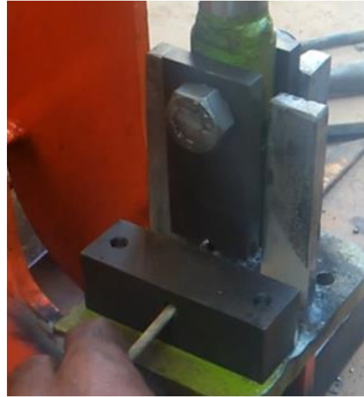
Fig. 2: Die manufactured for cutting of solid rods
