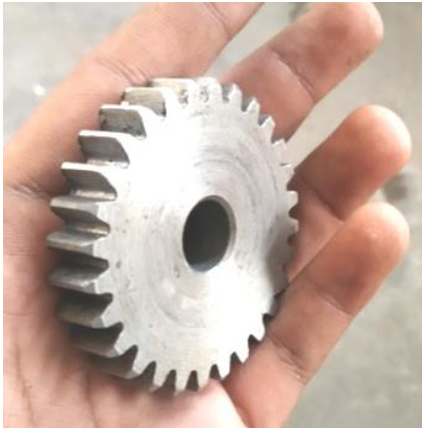
Fig. 3: Gear used for the rack and pinion
