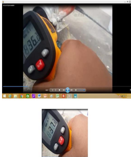
Fig 15 Temperature of tile cutter in working condition
