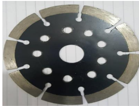
Fig 12 Optimised tile cutter
