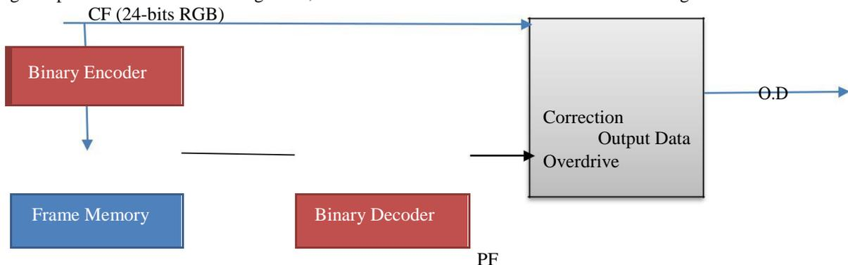
Fig.1 Basic block Diagram of LCD Overdrive
