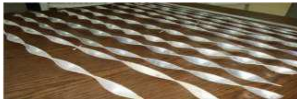
Figure-4: Twisted tape inserts [11]
