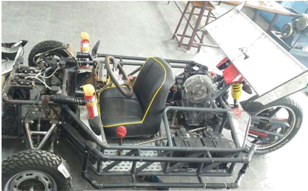
Fig- 7: Clear view of the vehicle and transmission system without solar panels
