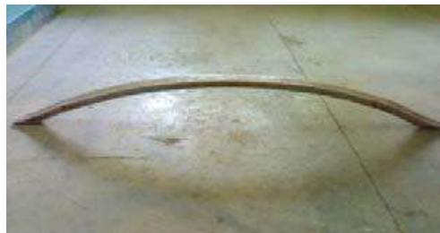
Fig2: Prepared Jute-Eglass-Epoxy composite leaf spring.
