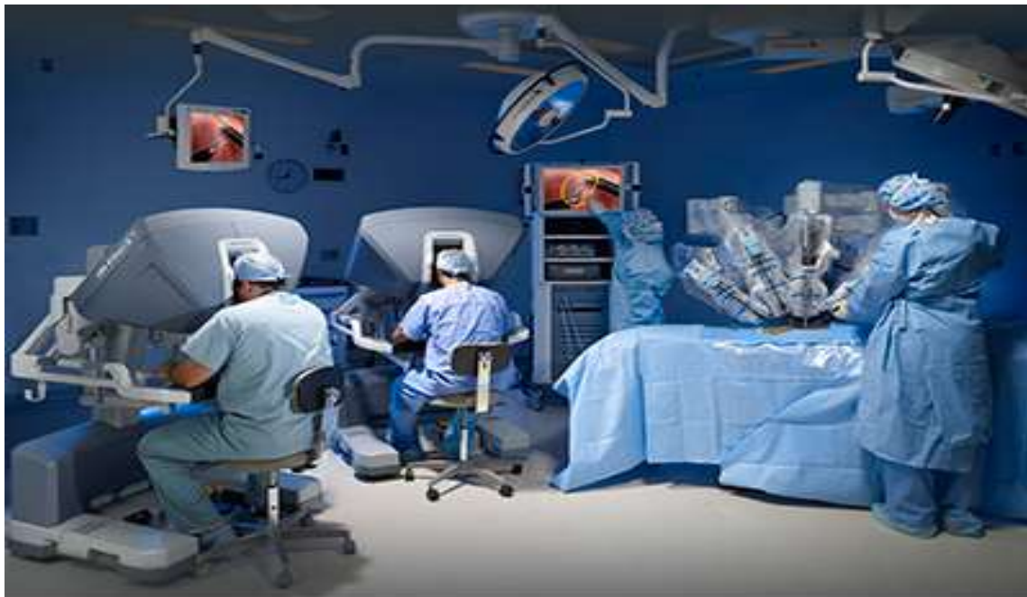
Teleoperated robot-assisted surgical system for minimally invasive procedures. (Credit: Intuitive Surgical, Inc.)
