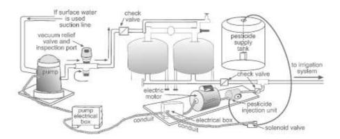
Minimum requirements for antipollution devices and arrangement of equipment for applying pesticides through an irrigation system using a pesticide injection unit powered by an electric motor and a media filtration system. (The same safety devices would be used by a system operating with an engine drive).
